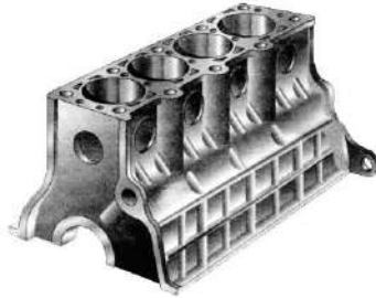
Figure 4.2 – Cylinder block of an inline four-cylinder engine
