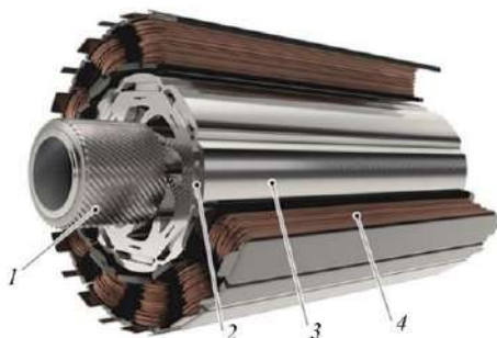
Figure 3.2 – Synchronous electric motor of an electric vehicle with permanent magnets: 1– gearbox drive gear; 2– permanent magnet gears; 3– rotor; 4– stator windings
