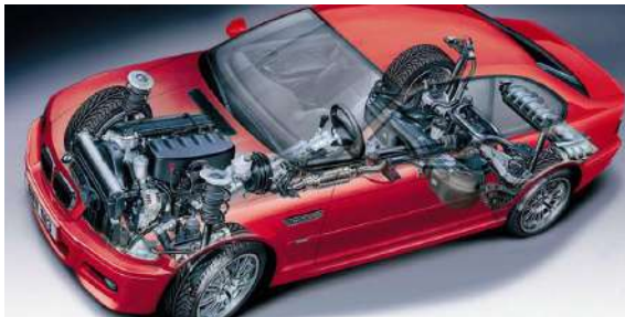
Figure 1.12 – Example of a classic passenger car layout car BMW
