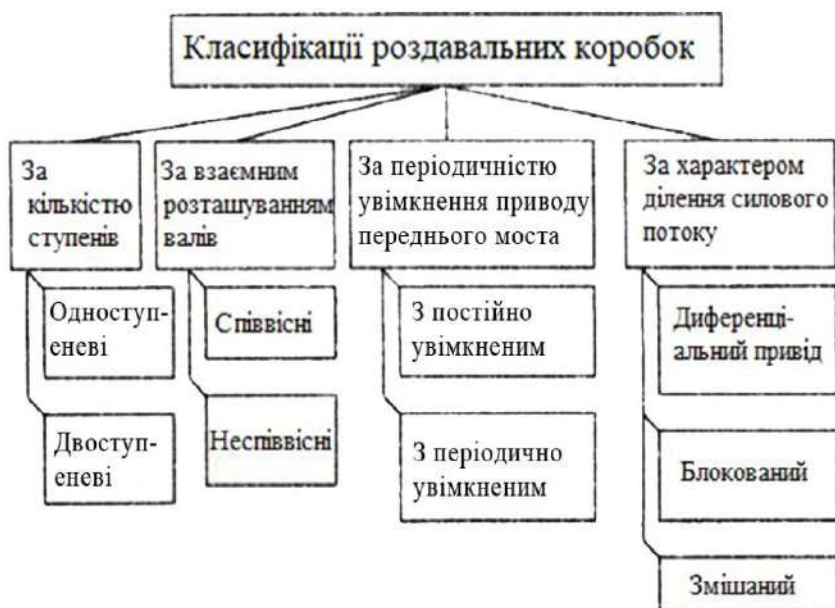
Figure 13.11 – Classification of transfer gearboxes
