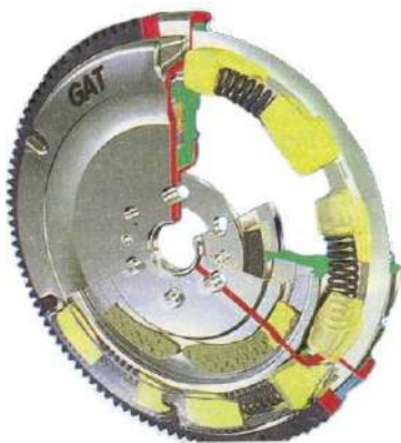
Figure 4.22 – Damping element, built into the flywheel
