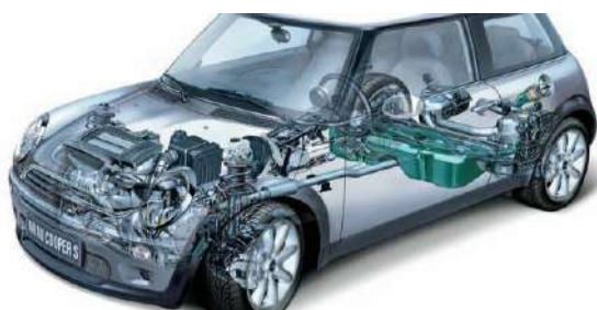
Figure 1.13 – Example of a front-wheel drive vehicle layout
