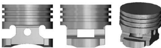
Figure 4.33 – X-shaped piston design
