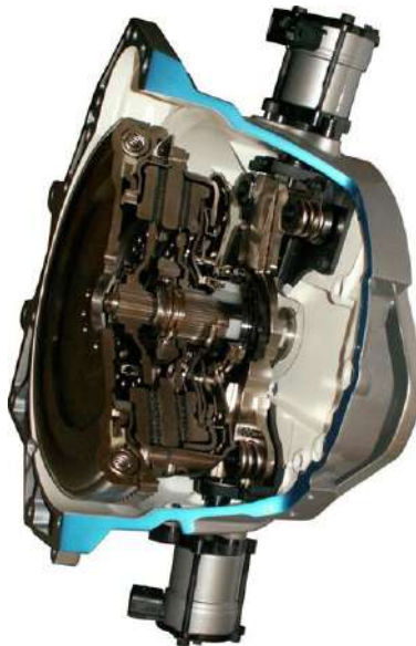
Figure 15.10 – Dry double clutch
