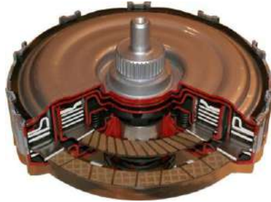
Figure 15.9 – Wet dual clutch
