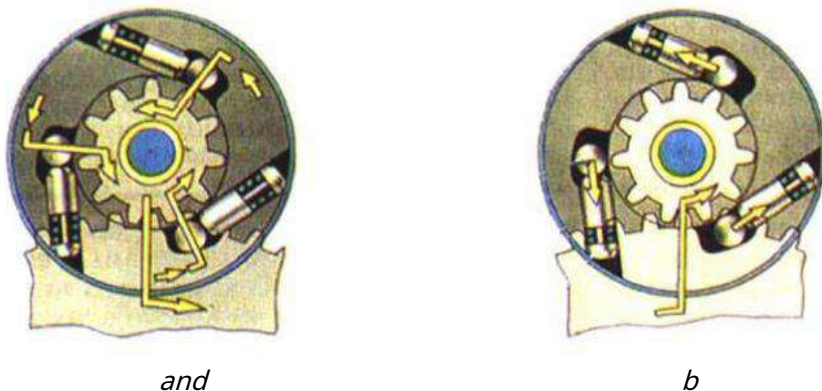
Figure 11.6 – Diagram of the operation of a roller overrunning clutch: at startup ( and ) and after start ( b ) car engine
