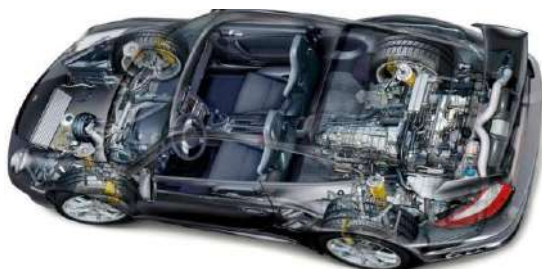
Figure 1.14 – Car with rear-engine powertrain layout unit
