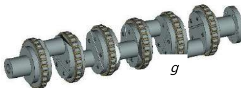
Figure 4.8 – Crankshafts: a – ZIL car engine130; b – YaMZ-236 diesel engine; in – KamAZ-740 diesel engine; g – design of a collapsible crank shaft (TATRA-815 car engine); 1– front end of the shaft; 2– dirt-catching cavity; 3– connecting rod neck; 4– counterweights; 5– oil deflector; 6– flange for fastening the flywheel; 7– root collar; 8 – cheek; 9– nut; 10 and 15– removable counterweights; 11– timing gear wheel; 12– installation pin; 13– drive gear wheel oil pump; 14– screw; 16– key; A – the amount of neck overlap
