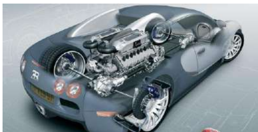
Figure 1.15 – Mid-engine all-wheel drive vehicle layout
