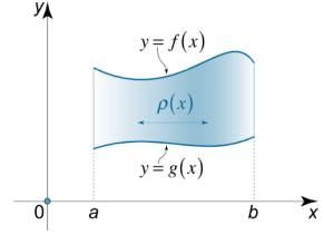
If the density of the lamina which occupies the region only depends on the x-coordinate, the total mass of the lamina is given by the integral
