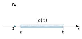
The density of the rod at any point x is defined by the density function  $\rho(x)$ . Assuming that  $\rho(x)$  is an integrable function, the mass of the rod is given by the integral.
