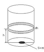
According to the law of Torricelli the speed of a liquid outflow is equal to  $v = k\sqrt{2gh}$ , where h – height of the liquid level above the hole. The amount of flowing out liquid at the time dt is equal to the volume  $\pi R^2 dh$ , where  $\pi R^2$  is an area of the cylinder basis. Then the speed of a liquid outflow through the hole with area  $S = \pi r^2$  will be equal
