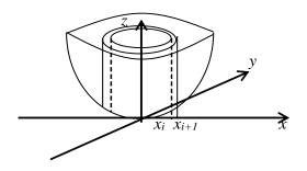
While solving the problems concerning calculation the inertia moment we should pay attention to the fact division on elementary subintervals should be carried out that all points of each selected segment should be approximately at similar distance from the rotation axis. In the given problem this can be achieved by division the paraboloid of gyration
