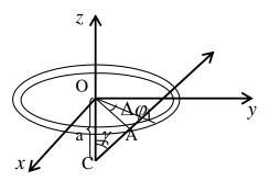
Here  $\rho$  – density function of weight,  $\Delta \varphi_i$ - angle, correspondent to the part of arch  $\Delta l_i$ (fig). Let's define the force  $\vec{F}_i$  of interaction of the material point *C* with the small segment of the ring  $\Delta l_i$ . For this let's decompose  $\vec{F}_i$  on basis  $\vec{i}, \vec{j}, \vec{k}$ .
