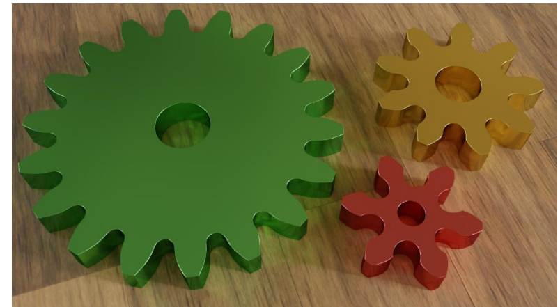
Gear with 20 teeth without undercut
