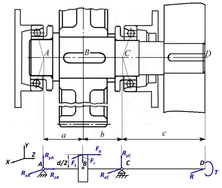
R - load on the shaft from a belt drive (Step 2 (15))
