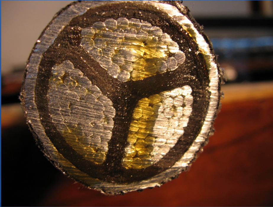
Cross section of a PILC (PIAC) cable sample from NPP
