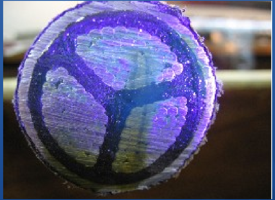
Cross section of a PILC (PIAC) cable sample from NPP
