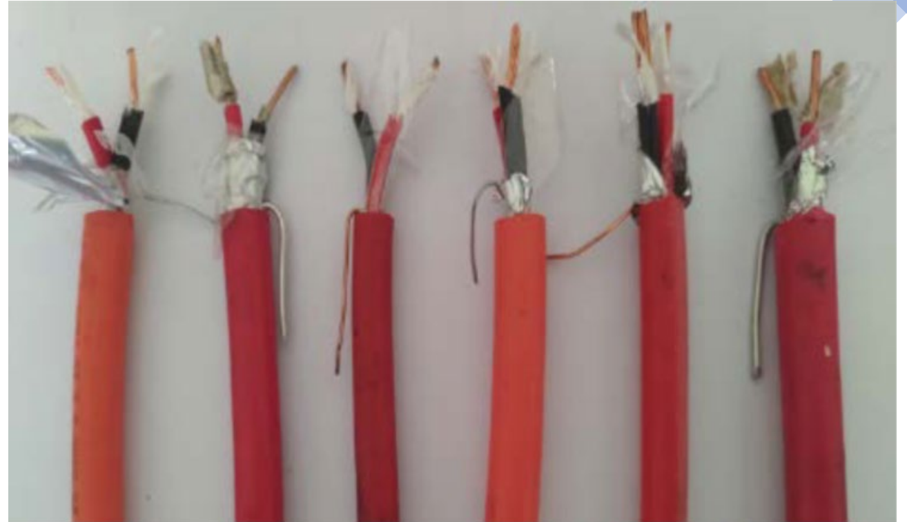
Fire-Resistant cables with mica/glass tape construction
