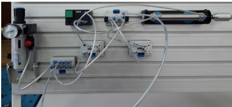
Fig. 3.12. Pneumatic circuit for speed control of a bilateral pneumatic cylinder based on 5/2 of the pneumatic distributor, implemented on "Festo" elements
