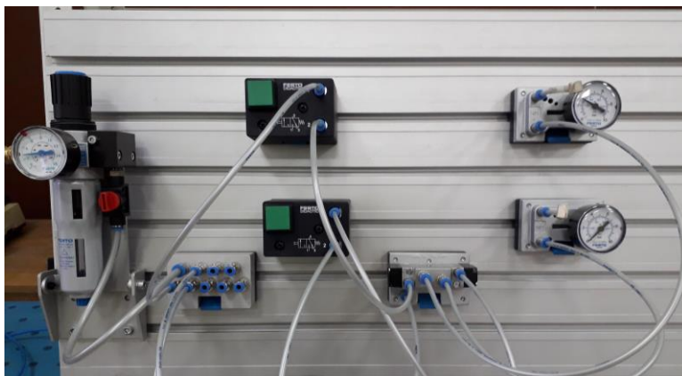
Fig. 1.10. Pneumatic diagram with memory elements implemented on "Festo" elements
