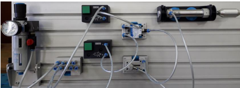
Fig. 1.35. Pneumatic scheme for the implementation of the function "And", implemented on the elements of "Festo"
