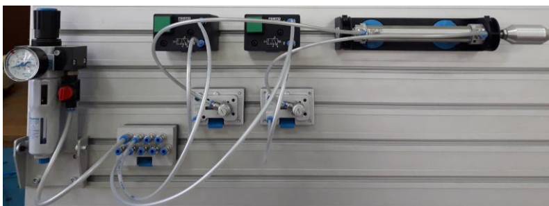
Fig. 3.10. Pneumatic circuit for speed control of a bilateral pneumatic cylinder based on 4/2 pneumatic distributor, implemented on "Festo" elements
