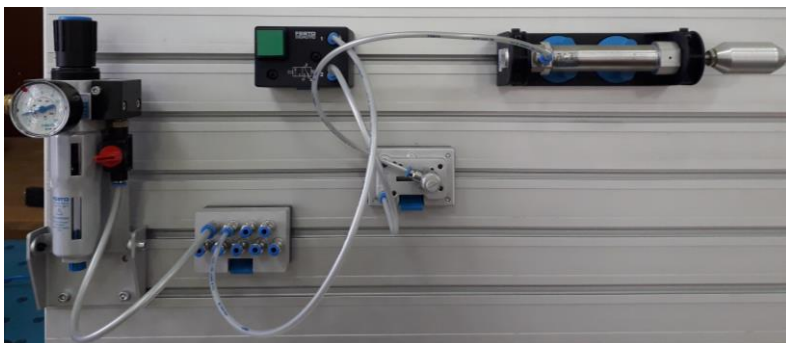
Fig. 3.4. Pneumatic scheme for speed control of a one-way pneumatic cylinder with spring return, implemented on "Festo" elements
