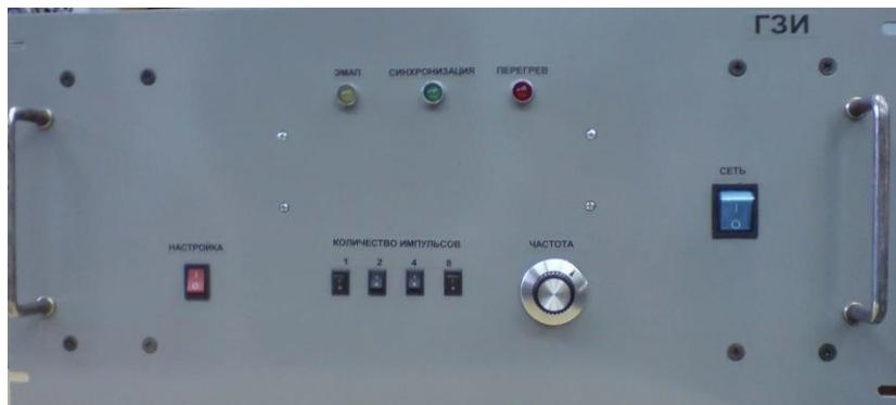
Probing pulse generator for automatic and mechanized installations for ultrasonic longitudinal inspection of metal products, shear, surface and normal waves
