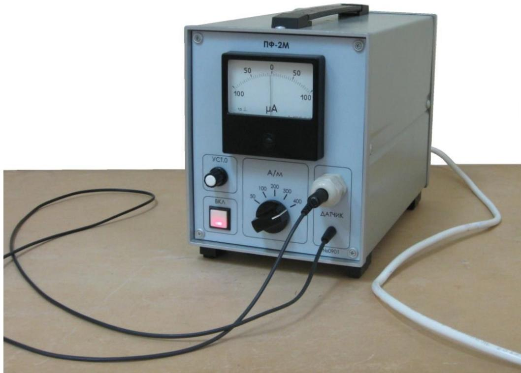
The PF-2M meter is designed to measure the intensity of stationary magnetic fields.
