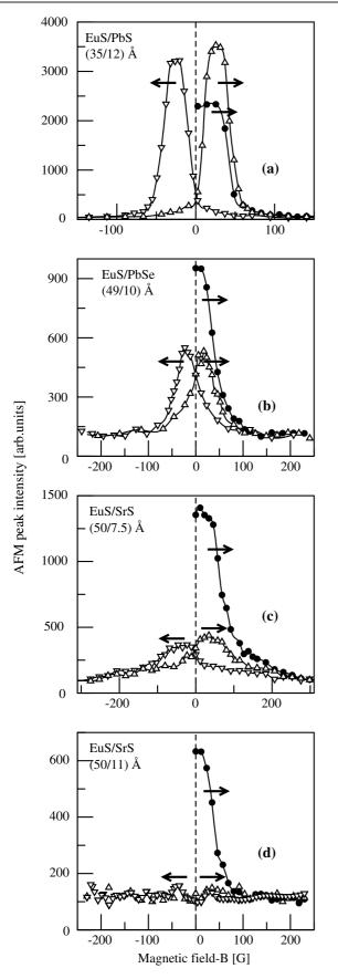
**Figure 3.** The intensity of the AFM SL Bragg peak versus sweeping magnetic field ('AFM hysteresis loops') for (a) EuS/PbS, (b) EuS/PbSe and (c), (d) EuS/SrS SLs. The direction of the field sweep is marked by the arrows.
