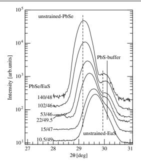
**Figure 7.** X-ray (200) reflection, measured in transmission geometry, from a number of pseudomorphic EuS/PbSe superlattices with approximately constant EuS and increasing PbSe layer thicknesses. Apart from the PbS buffer peak, there is only one maximum, which confirms the coincidence of the in-plane lattice parameters of EuS and PbSe. The value of the common in-plane lattice parameter shifts towards the unstrained (bulk) PbSe lattice constant as the thickness of the PbSe layer increases.
