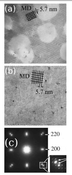
**Figure 8.** (a) Electron microscopy image of the Stransky–Krastanov mode of growth (island-like) of a thin PbTe layer on EuS; (b) electron microscopy image of the EuS–PbTe bilayer demonstrating the long range square misfit dislocation grid for the thicker, continuous, layers; (c) electron diffraction showing the satellites, accompanying the fundamental (200) and (220) reflections (see the arrows in the inset), arising from the periodic arrangement of dislocation lines at the interface.
