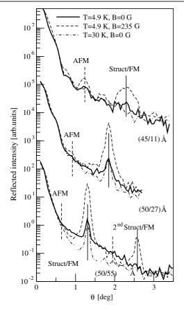
**Figure 5.** Unpolarized neutron reflectivity profiles taken below and above EuS Curie temperature ( $T_{\rm C} = 16.6$  K) in zero and saturating (235 G) magnetic field for three EuS/PbTe samples with different thicknesses of the nonmagnetic spacer PbTe.
