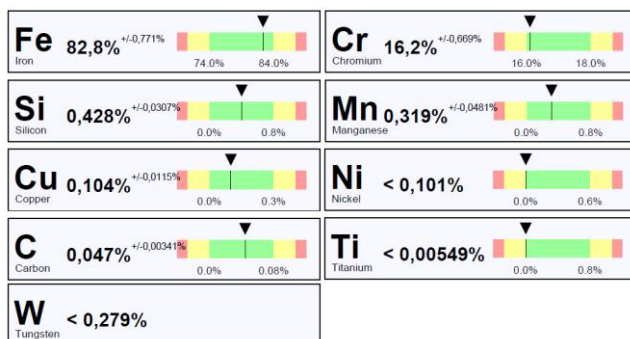
Figure 1. Chemical composition of the AISI 430 stainless steel substrates.
