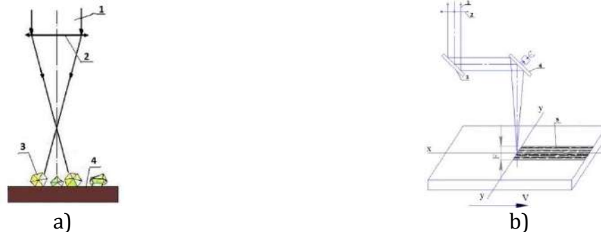
Figure 1. – Separation of abrasive material: a – by continuous or pulsed laser radiation; b – by scanning laser radiation.
