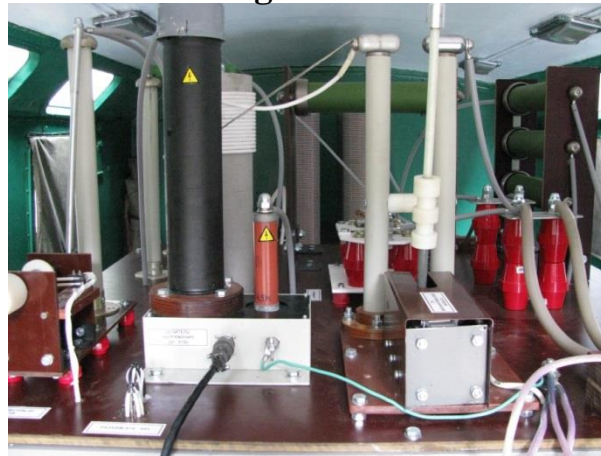
Installation "GIT-20" for the treatment of metallurgical sludge's
